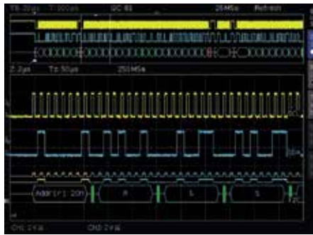
SPI bus signal, MISO / MOSI decoded
