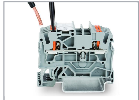
Insert fine-stranded conductors via operating tool.
