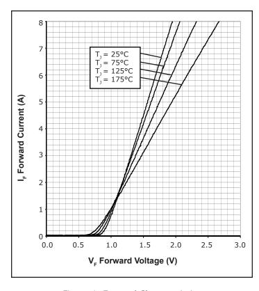
Figure 1. Forward Characteristics
