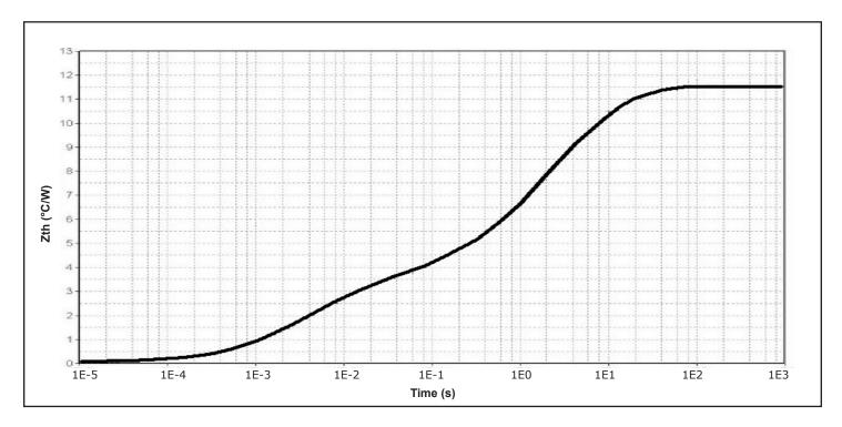
Figure 5. Transient Thermal Impedance
