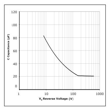
Figure 4. Capacitance vs. Reverse Voltage
