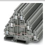
Multi-level terminal block, connection method: Screw connection, cross section: 0.14 mm² - 4 mm², AWG: 26 - 12, width: 5.2 mm, color: gray, mounting type: NS 35/7,5, NS 35/15
