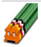
Feed-through terminal block, Connection method: Screw connection, Cross section: 0.14 mm<sup>2</sup> - 6 mm<sup>2</sup>, AWG: 26 - 10, Width: 6.2 mm, Color: red, Mounting type: NS 35/7,5, NS 35/15
