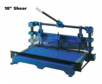
A bench top shear with an 18" (457mm) cutting capacity suitable for cutting printed circuit board laminates, thin metal sheet and aluminium (1.5/2.0mm) or plastic labels / front panel materials. On lowering the operating handle, a spring loaded clamp is activated which holds the material securely during cutting, thus enabling cuts to be made with a minimum of effort.
