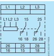
Connection diagram CM-MPS.31 and CM-MPS.41
