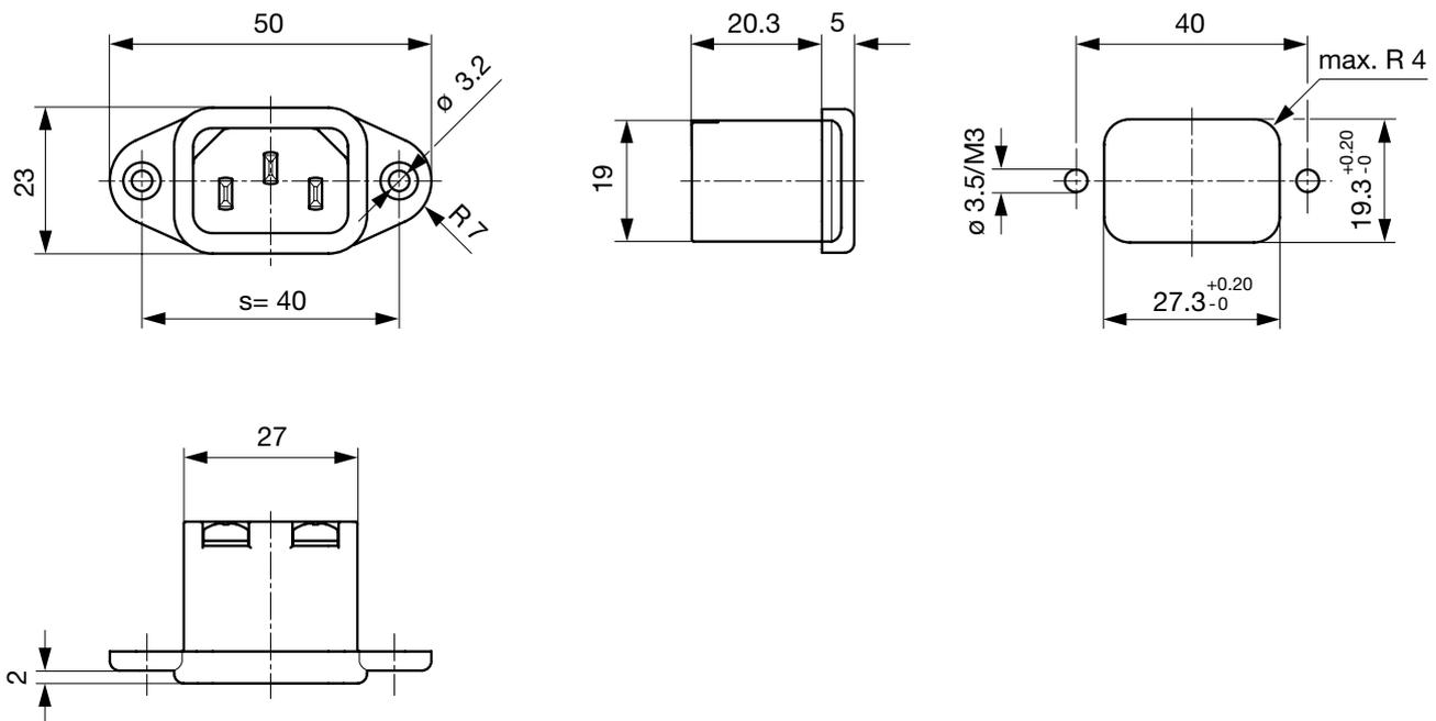
Protection class II, countersunk mounting holes, 40 mm distance, quick connect and solder terminals
