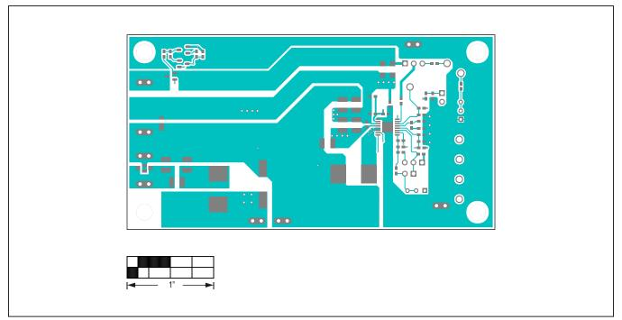
MAX25610 EV Kit PCB Layout—Top View
