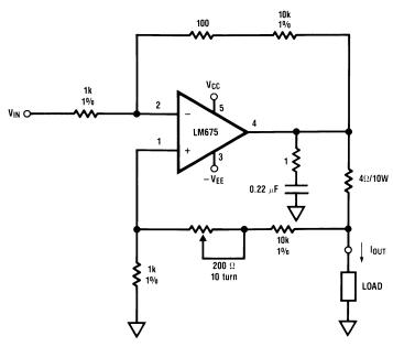
$$\begin{split} I_{OUT} &= V_{IN} \times 2.5 \text{ amps/volt} \\ \text{i.e. } I_{OUT} &= 1\text{A when } V_{IN} = 400 \text{ mV} \\ \text{Trim pot for max } R_{OUT} \end{split}$$
