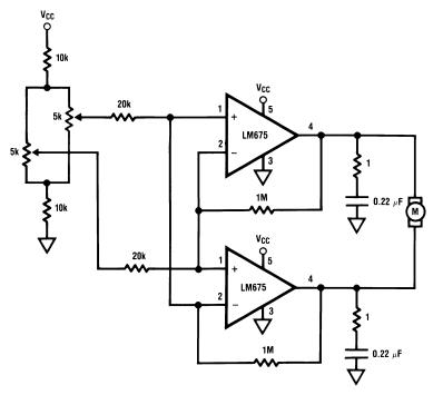
Figure 14. Servo Motor Control
