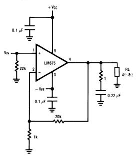
Figure 2. Non-Inverting Amplifier
