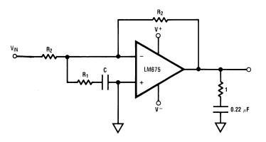
$$\begin{aligned} R_1C &\geq \frac{1}{2\pi500 \text{ kHz}} \\ R_1 &\leq \frac{R_2}{10} \\ A_{V(DC)} &= -1 \\ \end{aligned}$$
