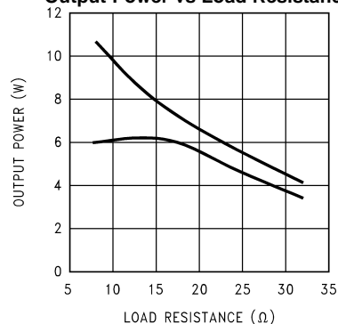
Figure 50. V_{DD} = 15V , BTL operation, f_{IN} = 1kHz , at (from top to bottom at 15Ω): THD+N = 10%, THD+N = 1%
