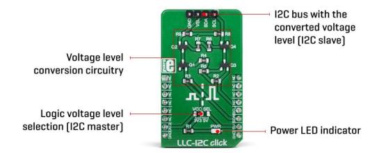
The I2C protocol was first introduced by NXP Semiconductors (formerly Philips Semiconductors), in 1982. They also introduced an application note that explains the operation of the LLC circuit in more details. The circuit is divided into *low-side* and *high-side* sections for future reference, although the circuit is symmetrical and can be used in both directions.
