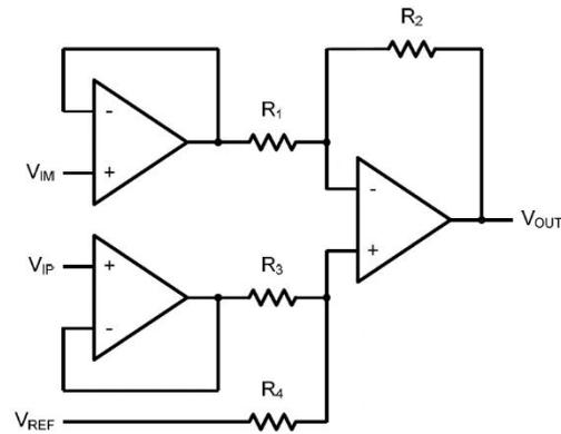
Figure 6. Instrument Amplifier
