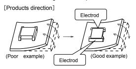
The electorode part of the products should be located like the picture to the mechanical stress.
