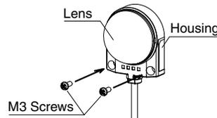
Note: The dome lens is not removable. Do not attempt to remove the lens, otherwise damage will occur.
