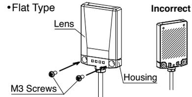
Note 1: Do not install the LH1D indicator by attaching only the lens, such as by taping down the lens. Otherwise internal components may come loose.
