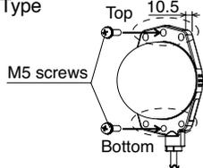
Note 1: Take into account the thickness of the base (10.5 mm), when selecting the length of the screws.
