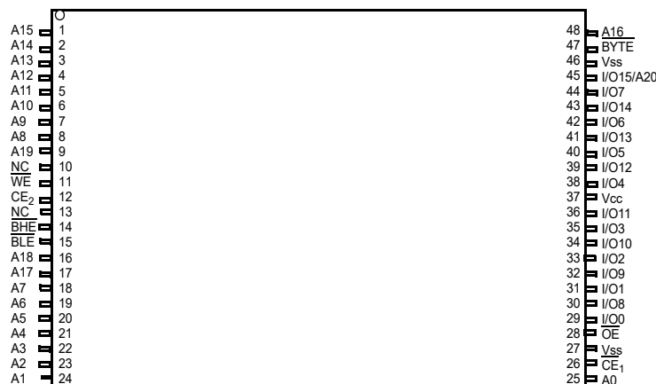
Figure 2. 48-pin TSOP I pinout (Top View) [2, 3]
