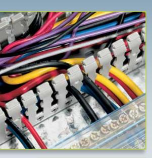
Transcab's durable PVC body consists of 6mm gaps and 6.5mm fingers with unique support ribs, providing strength and rigidity. Fingers are easily removed by snapping at support rib or base level to create T-junctions without the need for a saw.
