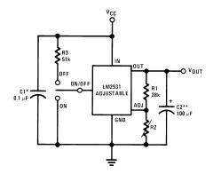
$V_{OUT} = \text{Reference Voltage} \times \frac{\text{R1} + \text{R2}}{\text{R1}}$
