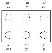
Figure 6. 6-Bump DSBGA Top View (Bump Side Down)
