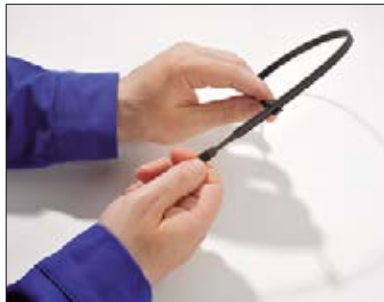
2. Pull the tie through the head until the bundle is fixed.
