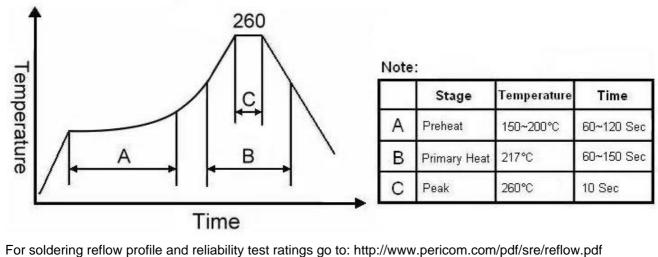
for soldering reflow profile and reliability test ratings go to: http://www.pericom.com/pdf/sre/reflow.pd
