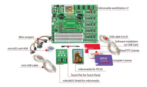
Each kit includes a mikromedia board, Visual TFT software license, compiler license, software installation on USB card, a mikroBUS Shield for mikromedia, mikromedia workStation v7, Touch pen for the screen, mini USB and USB type A to B cable, microSD card (4GB), and 30 pieces of wire jumpers.
