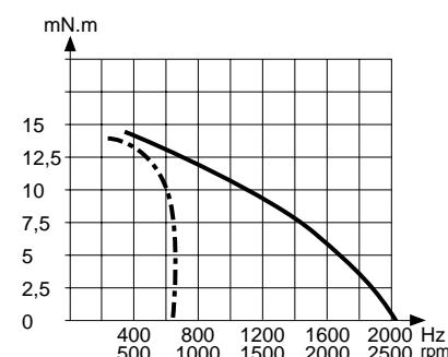
**4 phases - 115 Ω - Constant voltage - Curve produced with card 84 854 405 (see p.3/21)**
