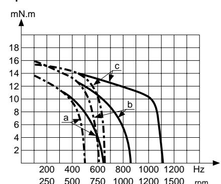
The measurements are made with full stepping, 2 phases energised.
