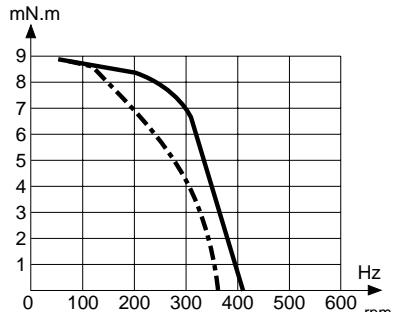
Max. stopping-starting and operating curves at I constant (PBL 3717) for 2 (motor) phases 12.9 ohms.
