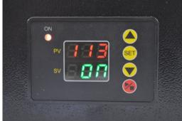
8. Once the timer has counted down to zero the UV tubes will be automatically switched off, and the display will display OFF. It is now safe to lift the "exposure top" and undo the catches of the clamp down frame to access the exposed work piece and remove the exposed part and artwork, the unit is then ready for the next part to be exposed. RED STOP/START
