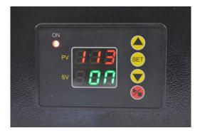
To set the exposure time with the display showing 000/OFF press the "SET" button twice in quick succession, the RED digits will then flash, and the digits on the display can be set to your required exposure time, for example 075 seconds by using the "UP" ■ and "DOWN" ■ arrow keys. When you have set the correct time, press the SET button twice, and timer will run through the "Pre Warm up" start up sequence.
