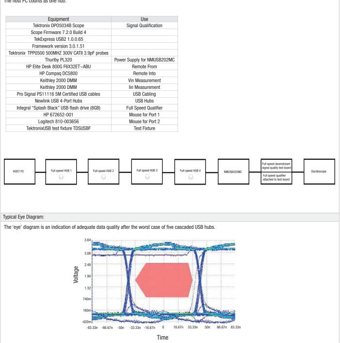
NMUSB202MC is equivalent to one USB hub for dynamic characteristics, verified by the setup in the figure below for worst case USB specification of 5 cascaded hubs. The host PC counts as one hub.
