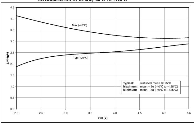
FIGURE 23-29: △IPD FSCM vs. VDD OVER TEMPERATURE PRI\_IDLE MODE, EC OSCILLATOR AT 32 kHz, -40°C TO +125°C
