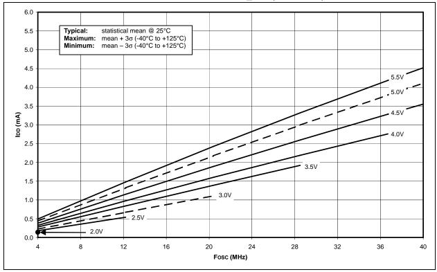
FIGURE 23-13: TYPICAL IDD vs. Fosc OVER VDD PRI\_IDLE, EC MODE, +25°C
