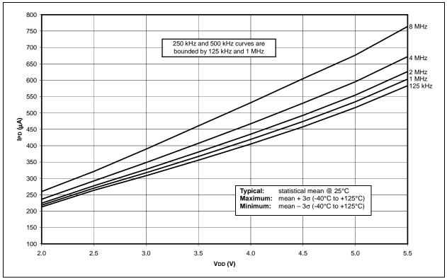
FIGURE 23-20: TYPICAL AND MAXIMUM IPD vs. VDD (-40°C TO +125°C), 31.25 kHz RC\_IDLE MODE, ALL PERIPHERALS DISABLED
