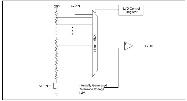
The LVD module has an additional feature that allows the user to supply the trip voltage to the module from an external source. This mode is enabled when bits, LVDL3:LVDL0, are set to '1111'. In this state, the comparator input is multiplexed from the external input pin, LVDIN (Figure 18-3). This gives users flexibility, because it allows them to configure the Low-Voltage Detect interrupt to occur at any voltage in the valid operating range.
