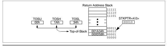
**Note:** Returning a value of zero to the PC on an underflow has the effect of vectoring the program to the Reset vector, where the stack conditions can be verified and appropriate actions can be taken. This is not the same as a Reset, as the contents of the SFRs are not affected.
