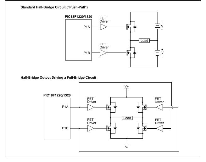
The TRISB<3:2> and TRISB<7:6> bits must be cleared to make the P1A, P1B, P1C and P1D pins output.
