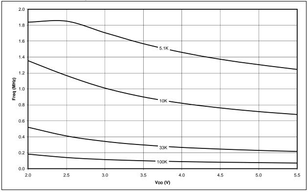
FIGURE 23-36: AVERAGE Fosc vs. VDD FOR VARIOUS R'S EXTERNAL RC MODE, C = 300 pF, TEMPERATURE = +25°C
