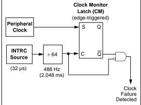
Clock failure is tested for on the falling edge of the sample clock. If a sample clock falling edge occurs while CM is still set, a clock failure has been detected (Figure 19-4). This causes the following:
