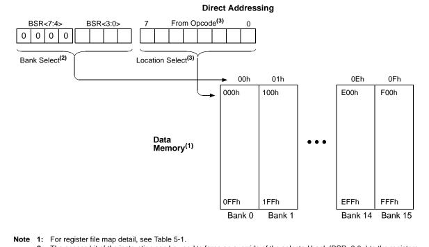
2: The access bit of the instruction can be used to force an override of the selected bank (BSR<3:0>) to the registers of the Access Bank.
