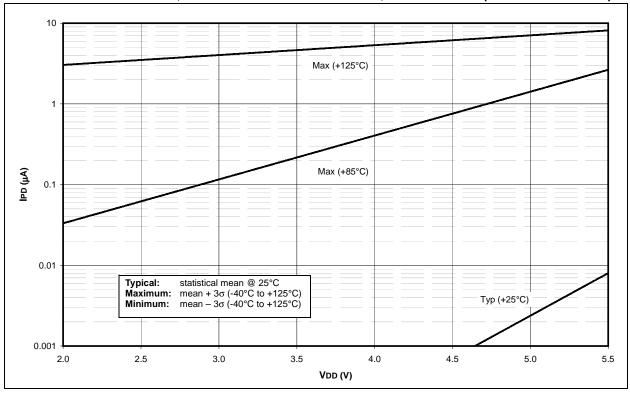
FIGURE 23-33: △IPD A/D, -40°C TO +125°C SLEEP MODE, A/D ENABLED (NOT CONVERTING)
