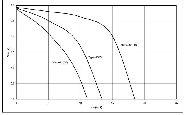
FIGURE 23-25: VOH vs. IOH OVER TEMPERATURE (-40°C TO +125°C), VDD = 5.0V
