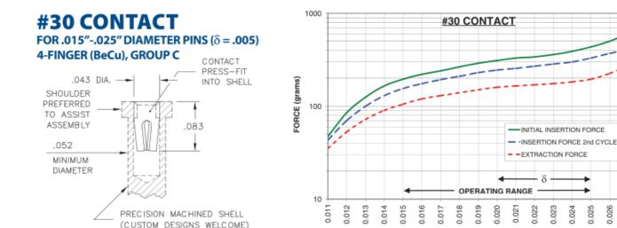
The insertion / extraction force characteristics above were derived using a 30 microinch gold-plated contact and polished steel gauge pins having a bullet-shaped tip. The curves represent typical average values; they are best used to compare the differences between similar size contacts and to guide you in selecting one that is suitable for your application. Your results may vary, so for your specification, we encourage you to obtain complimentary samples for your evaluation.
