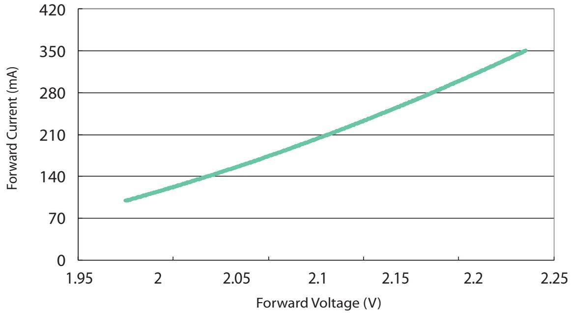
Forward Current vs. Forward Voltage for 1W Cyan
