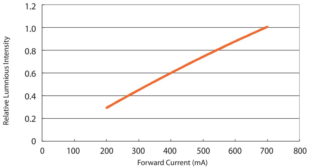
Relative Luminous Intensity vs. Forward Current for 3W Amber
