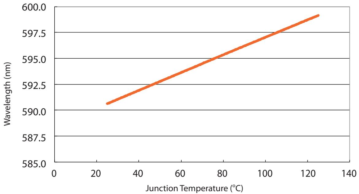
Wavelength vs. junction temperature for 3W Amber
