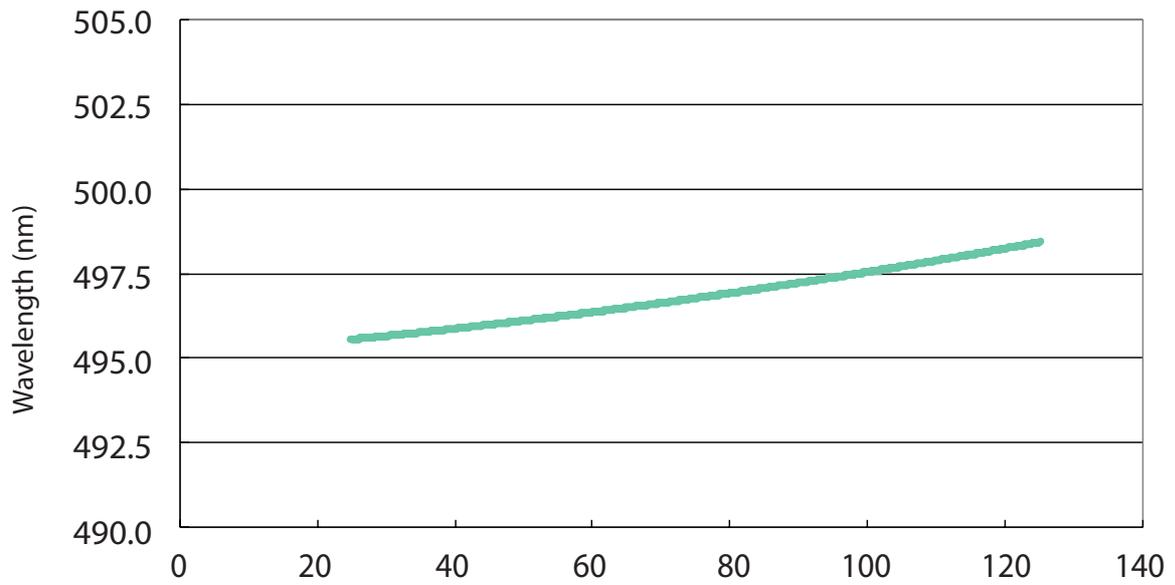
Wavelength vs. junction temperature for 1W Cyan
