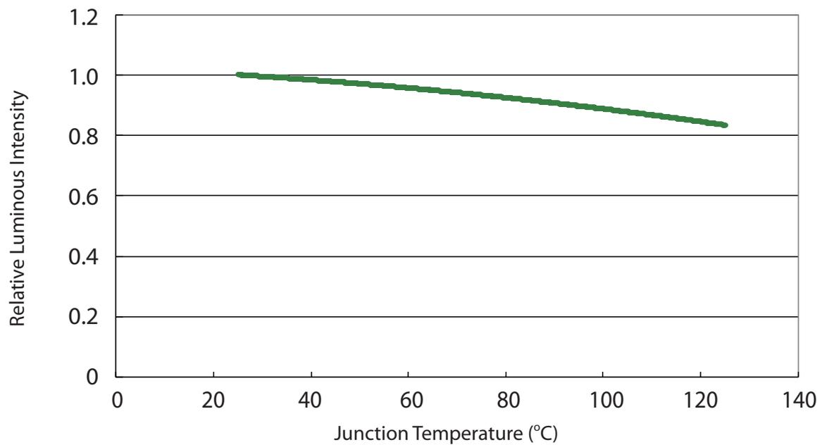
Relative Luminous Intensity vs. junction temperature for 3W True Green
