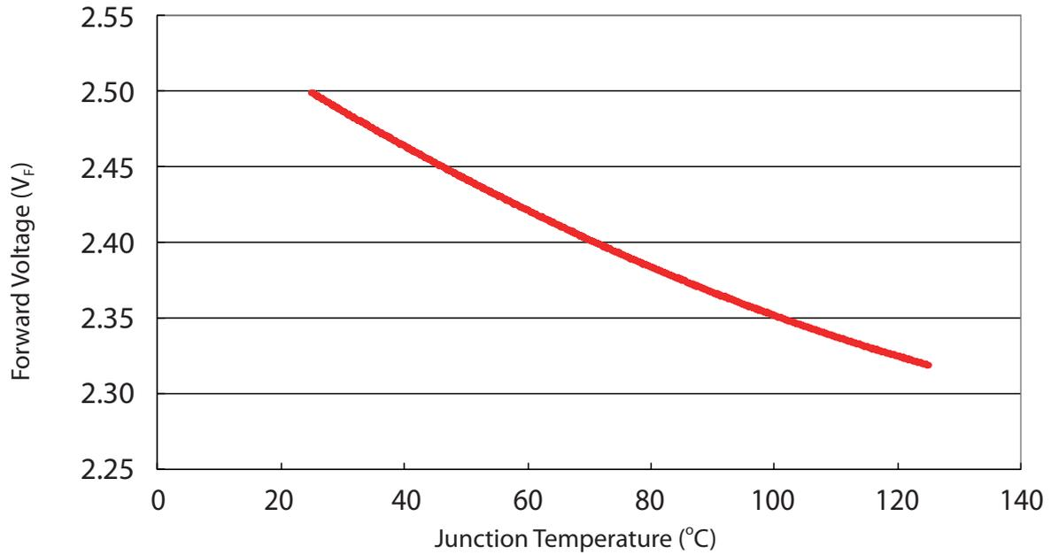
Forward voltage vs. junction temperature for 3W Red
