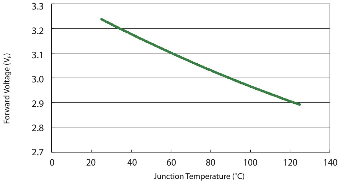
Forward voltage vs. junction temperature for 1W True Green
