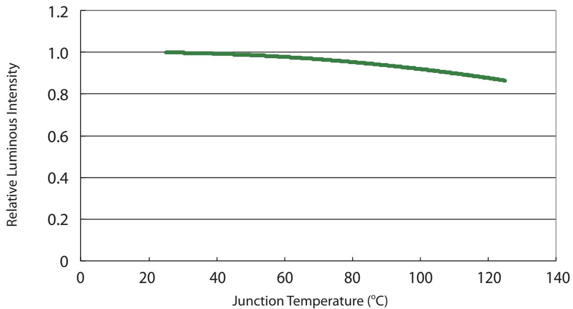
Relative Luminous Intensity vs. junction temperature for 1W True Green
