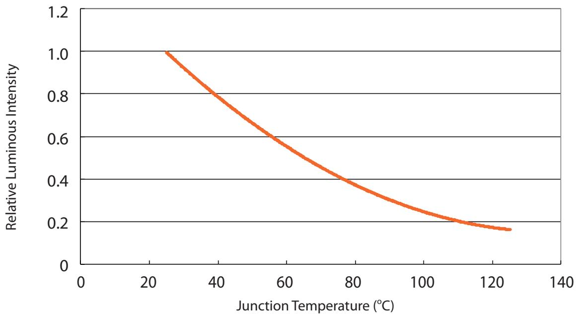
Relative Luminous Intensity vs. junction temperature for 3W Amber
