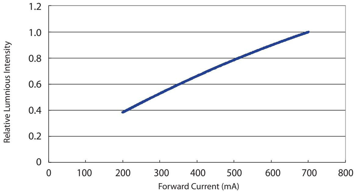
Relative Luminous Intensity vs. Forward Current for 3W Blue
