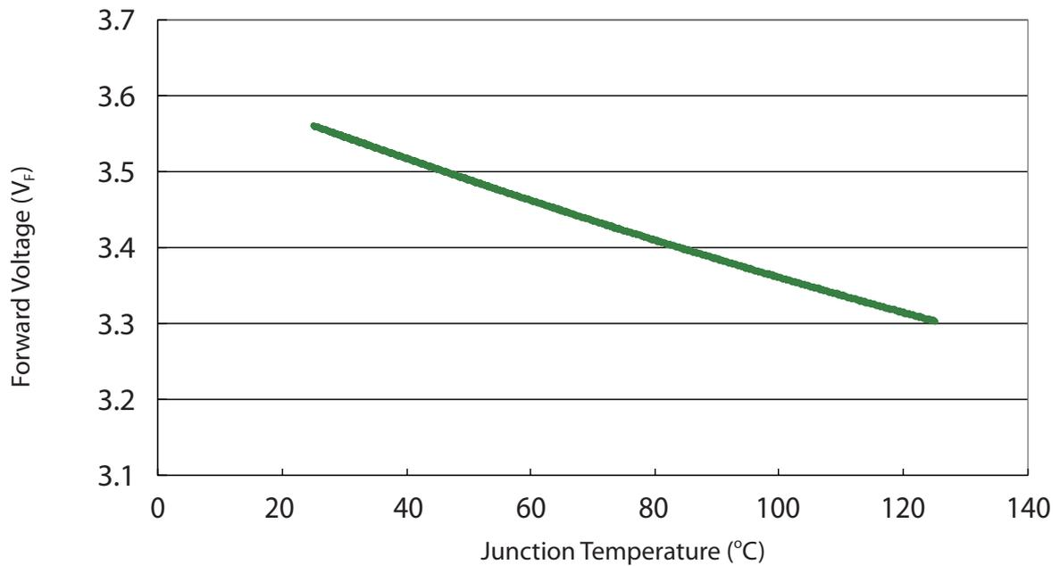
Forward voltage vs. junction temperature for 3W True Green
