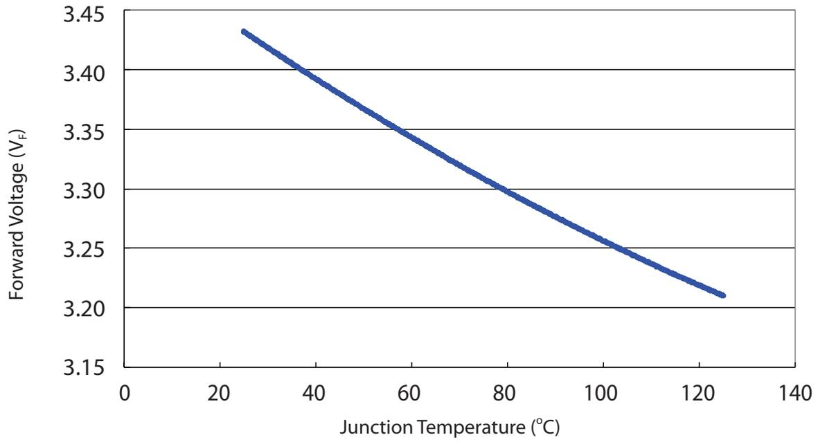
Forward voltage vs. junction temperature for 3W Dental Blue
