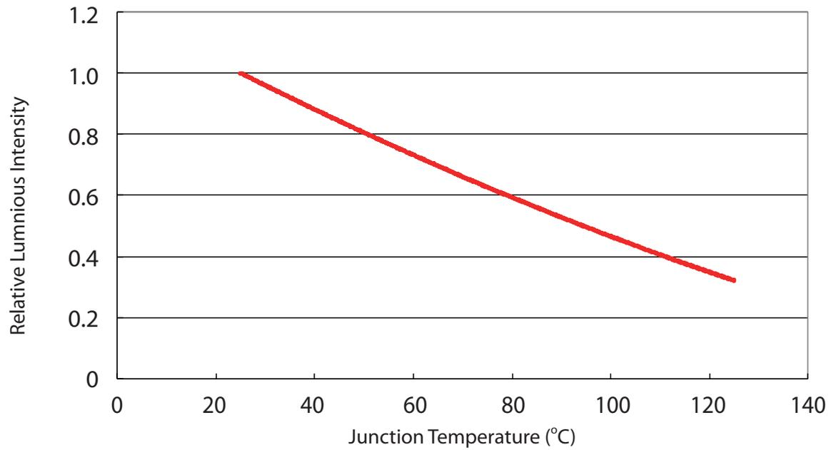
Relative Luminous Intensity vs. junction temperature for 3W Red
