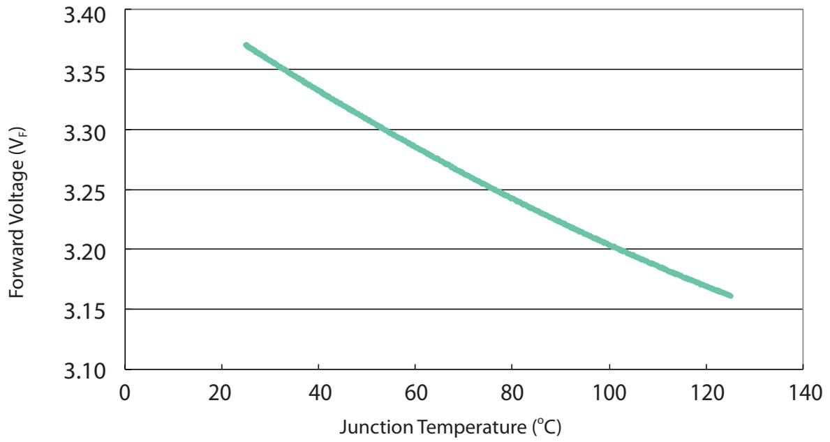
Forward voltage vs. junction temperature for 1W Cyan
