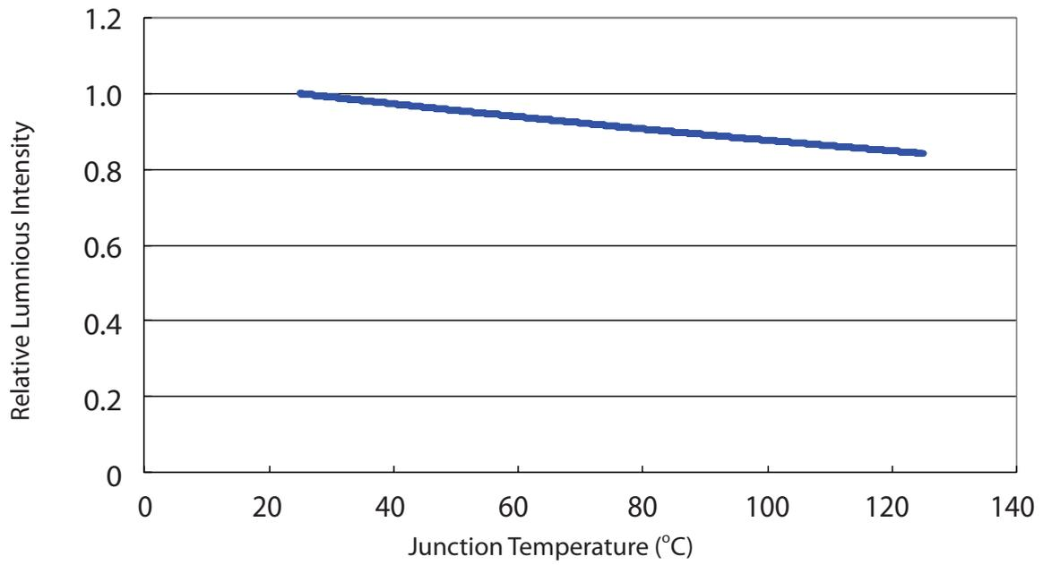
Relative Luminous Intensity vs. junction temperature for 3W Dental Blue
