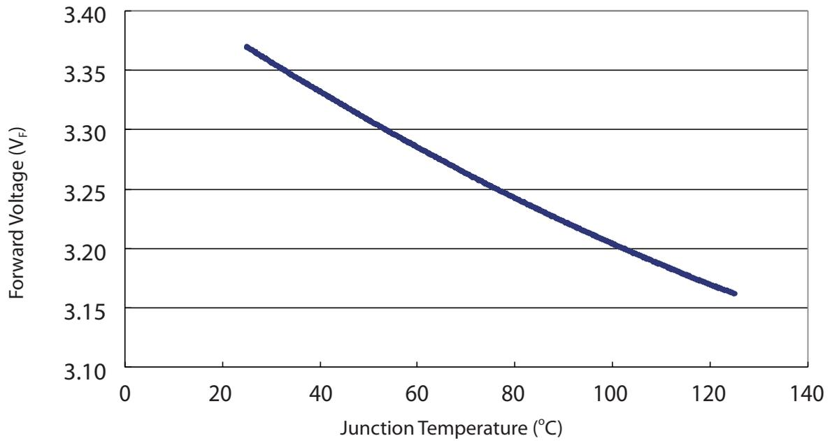
Forward voltage vs. junction temperature for 1W Blue
