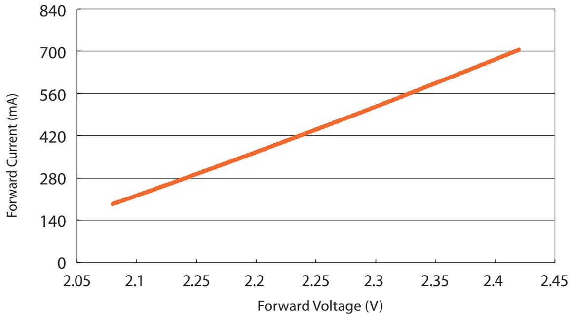
Forward Current vs. Forward Voltage for 3W Amber
