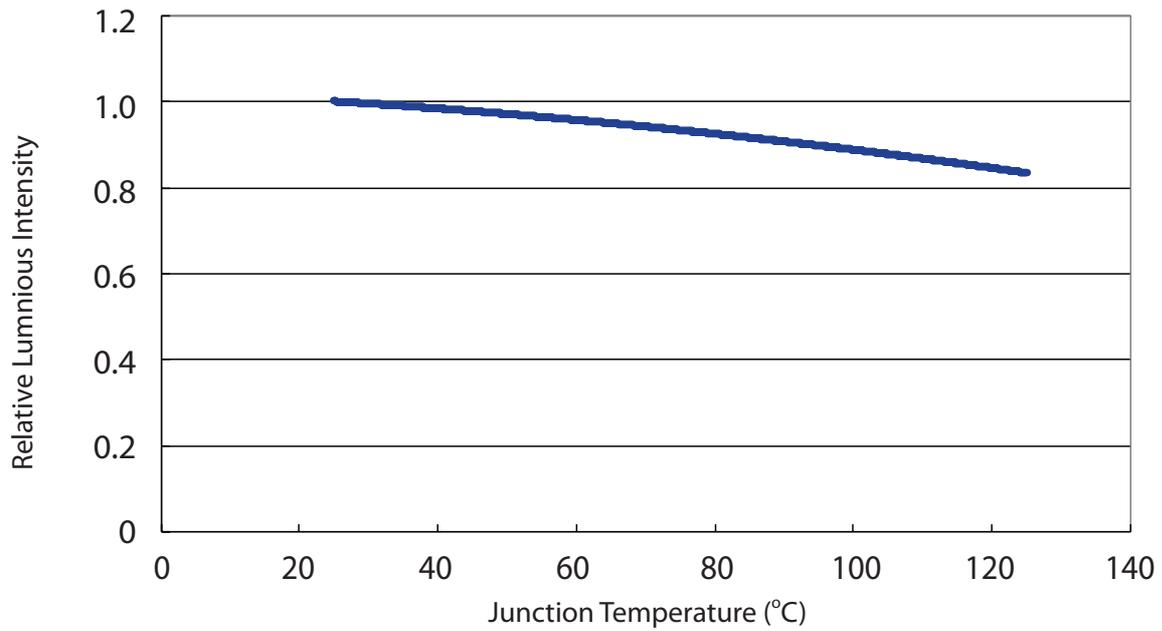
Relative Luminous Intensity vs. junction temperature for 3W Blue
