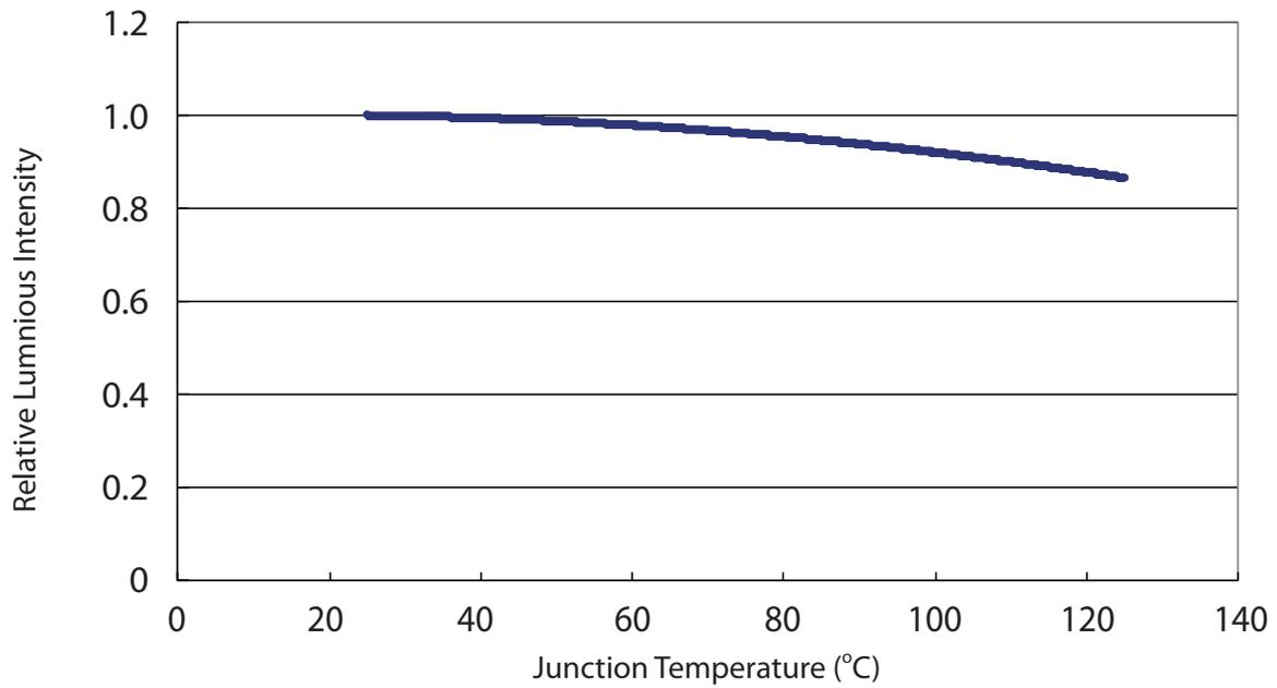
Relative Luminous Intensity vs. junction temperature for 1W Blue
