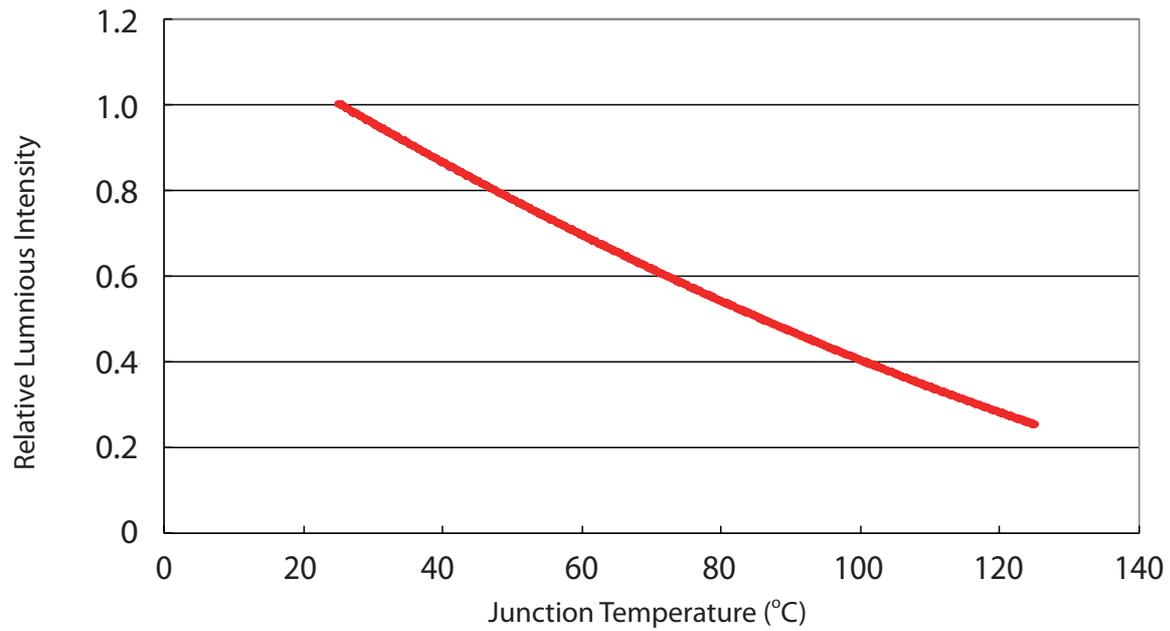
Relative Luminous Intensity vs. junction temperature for 1W Red
