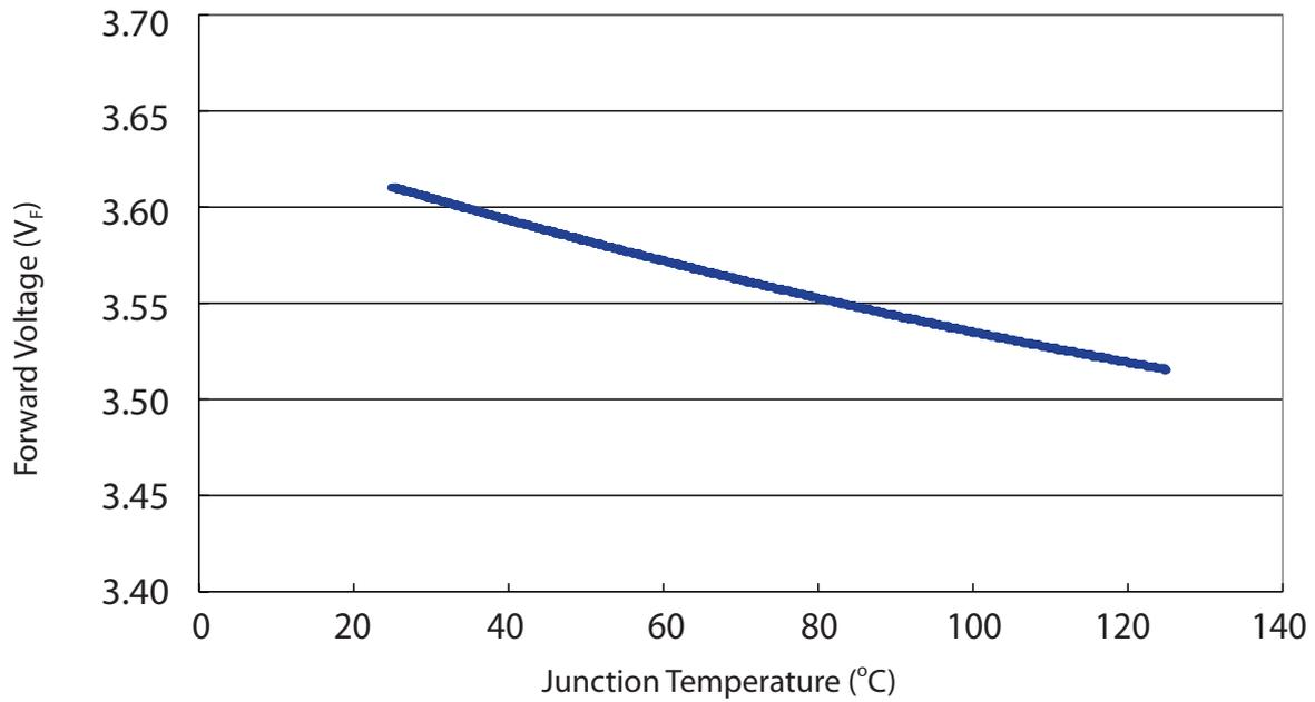
Forward voltage vs. junction temperature for 3W Blue
