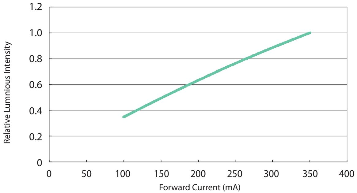
Relative Luminous Intensity vs. Forward Current for 1W Cyan
