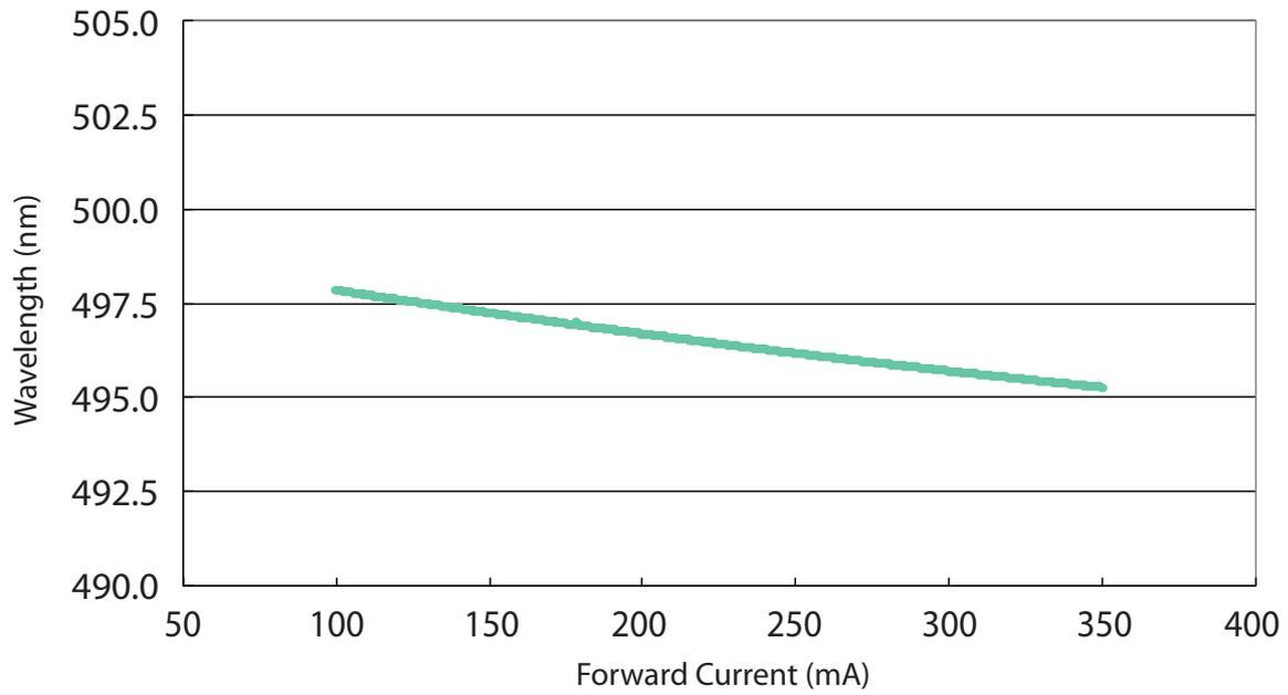
Wavelength vs. Forward Current for 1W Cyan
