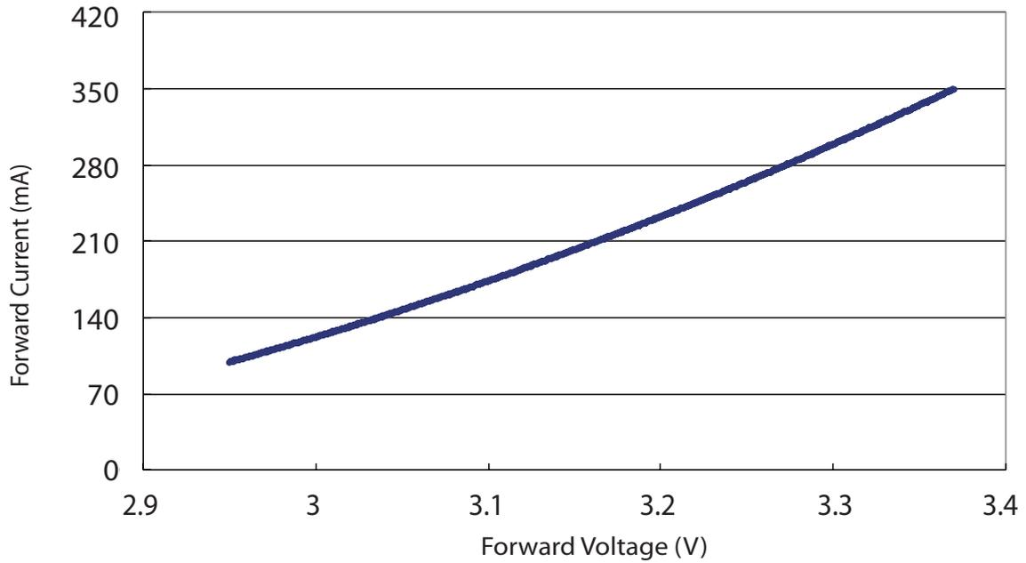
Forward Current vs. Forward Voltage for 1W Blue
