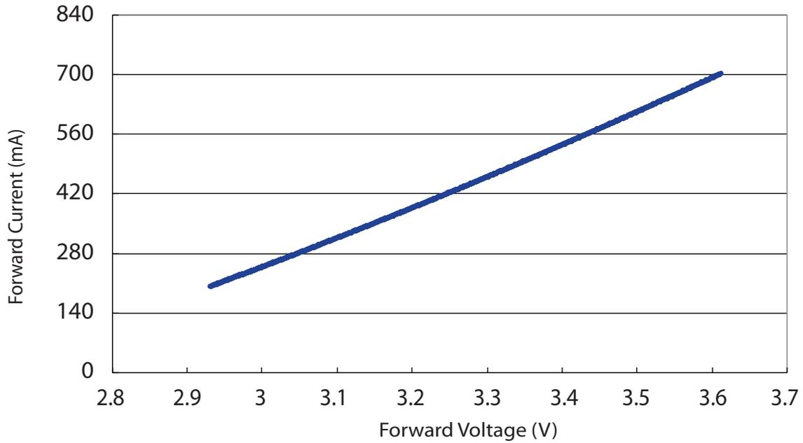
Forward Current vs. Forward Voltage for 3W Blue
