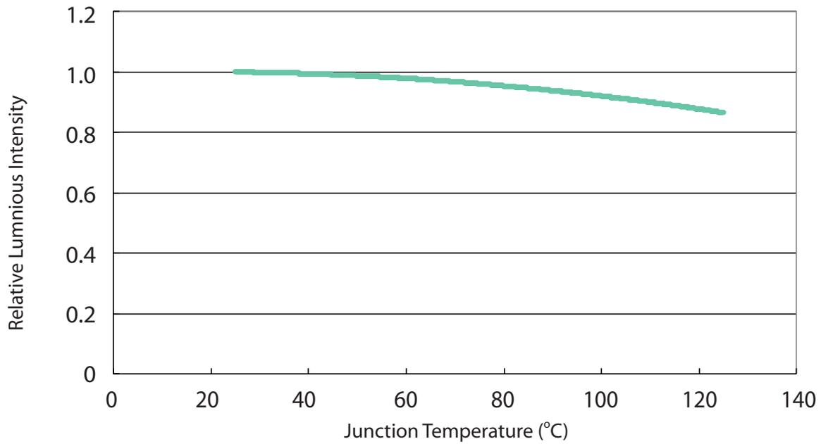
Relative Luminous Intensity vs. junction temperature for 1W Cyan
