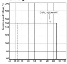
Ambient temperature (°C) Note The "maximum coil voltage" is the maximum voltage that can be applied to the Relay coil.
