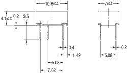
Note: Each value has a tolerance of ±0.3 mm.
