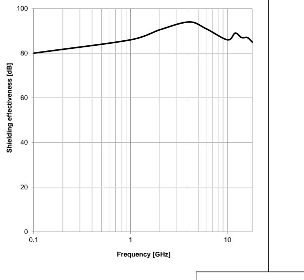
CHECKED REVISION DATE (YYYY-MM-DD) GENERAL TOLERANCE PROJECTION METHOD ViMa 005.003 2020-03-06 DIN ISO 2768-1m DESCRIPTION **WE-LT Conductive Shielding** Würth Elektronik eiSos GmbH & Co. KG Gasket ORDER CODE EMC & Inductive Solutions Max-Eyth-Str. 1 3021003 74638 Waldenburg Germany SIZE/TYPE STATUS Tel. +49 (0) 79 42 945 - 0 www.we-online.com BUSINESS UNIT PAGE WÜRTH ELEKTRONIK 2/3 eiSos Valid Square eiSos@we-online.com
