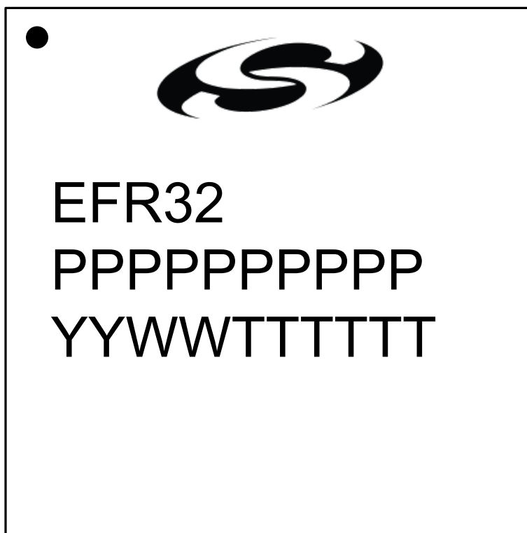
Figure 7.3. BGA125 Package Marking
