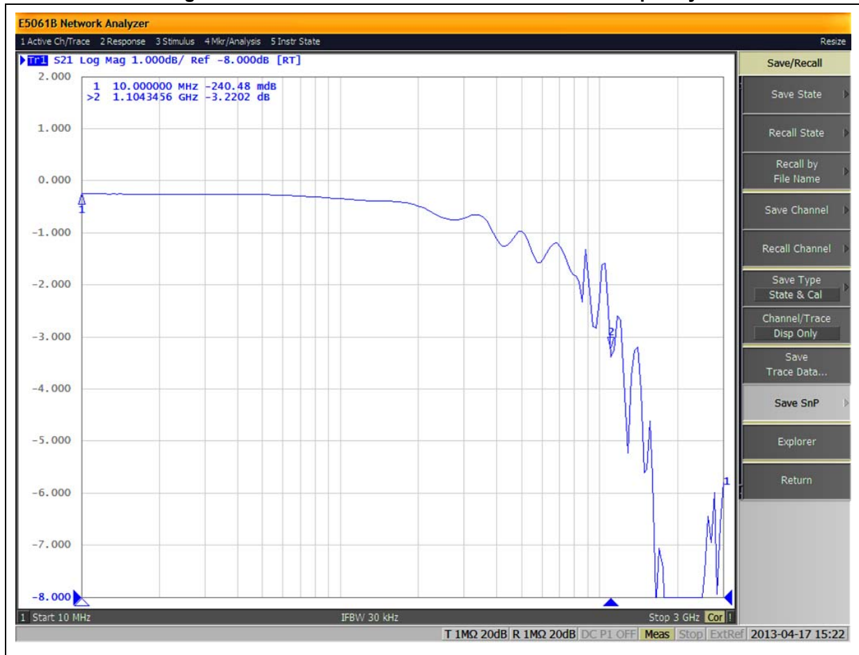
Figure 17. Data switch transfer characteristics vs. frequency
