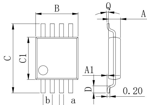
Dimensions In Millimeters(MSOP8L)
