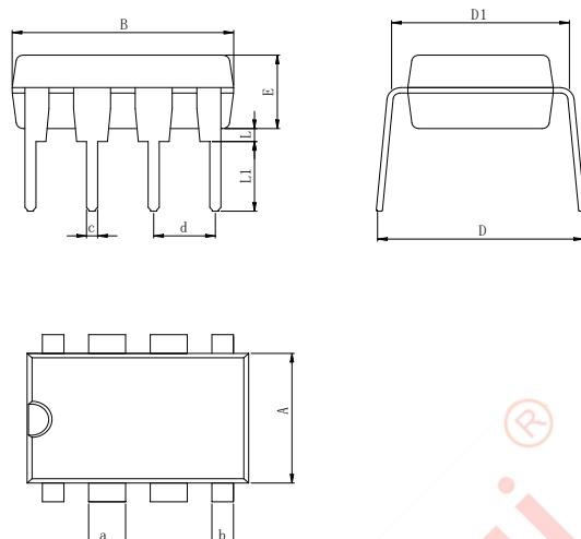
Dimensions In Millimeters(DIP8L)
