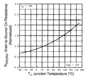
Fig. 4 - Normalized On-Resistance vs. Temperature
