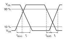
Fig. 10b - Switching Time Waveforms
