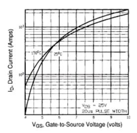
Fig. 3 - Typical Transfer Characteristics
