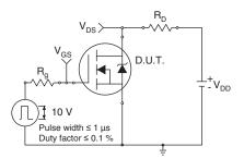
Fig. 10a - Switching Time Test Circuit
