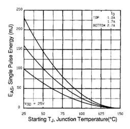
Fig. 12c - Maximum Avalanche Energy vs. Drain Current
