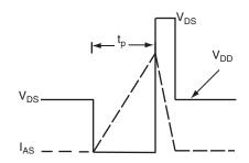
Fig. 12b - Unclamped Inductive Waveforms
