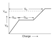
Fig. 13a - Basic Gate Charge Waveform
