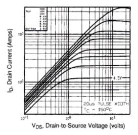
Fig. 2 - Typical Output Characteristics,  $T_C = 150 \, ^{\circ}C$
