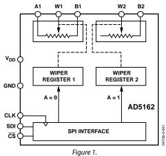
Operating from a 2.7 V to 5.5 V power supply and consuming less than 6  $\mu$ A allows the AD5162 to be used in portable battery-operated applications.
