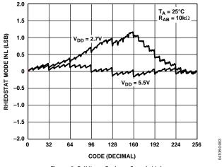
Figure 3. R-INL vs. Code vs. Supply Voltages
