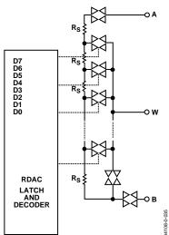
Figure 34. AD5162 Equivalent RDAC Circuit
