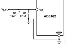
Figure 39. Power Supply Bypassing
