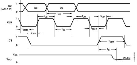
Figure 43. SPI Interface Detailed Timing Diagram ( $V_A = 5 V$ ,  $V_B = 0 V$ ,  $V_W = V_{OUT}$ )
