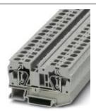
Feed-through terminal block, Connection method: Spring-cage connection, Cross section: 0.2 mm² - 10 mm², AWG: 24 - 8, Width: 8.2 mm, Color: gray, Mounting type: NS 35/7,5, NS 35/15
