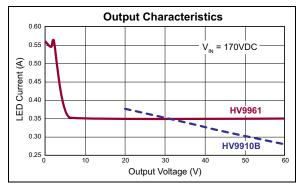
FIGURE 3-1: Typical Output Characteristic of an HV9961 LED Driver.
