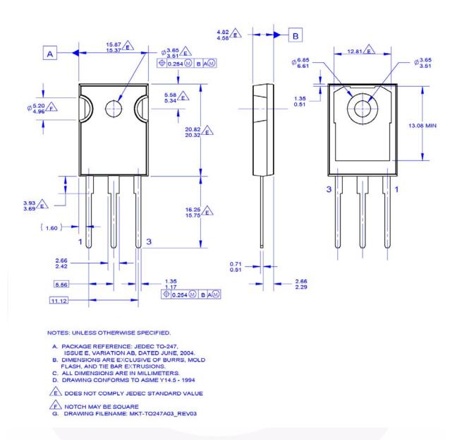
Figure 20. TO-247 3L - TO-247, MOLDED, 3 LEAD, JEDEC VARIATION AB
