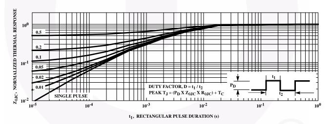
FIGURE 17. NORMALIZED TRANSIENT THERMAL RESPONSE, JUNCTION TO CASE
