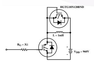
FIGURE 18. INDUCTIVE SWITCHING TEST CIRCUIT
