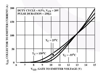
FIGURE 13. TRANSFER CHARACTERISTIC
