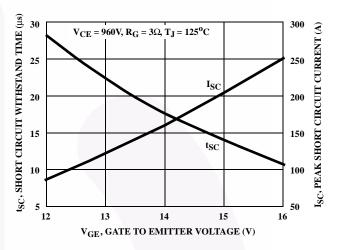
FIGURE 4. SHORT CIRCUIT WITHSTAND TIME
