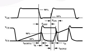
FIGURE 19. SWITCHING TEST WAVEFORMS
