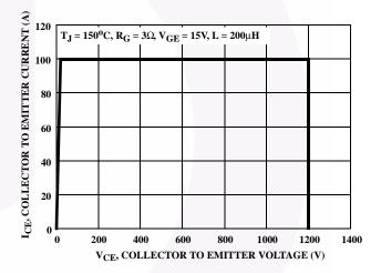
FIGURE 2. MINIMUM SWITCHING SAFE OPERATING AREA
