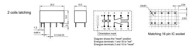
Remark: 1) In case of no tolerance shown in outline dimension: outline dimension ≤1mm, tolerance should be ±0.2mm; outline dimension >1mm and ≤5mm, tolerance should be ±0.3mm; outline dimension >5mm, tolerance should be ±0.4mm.
