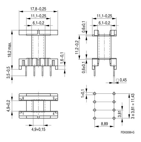
Hole arrangement View in mounting direction
