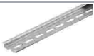
Item no.: 210-115 Steel carrier rail; 35 x 7.5 mm; 1 mm thick; 2 m long; slotted; according to EN 60715; "Hole width 18 mm; silver-colored
