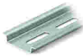
Item no.: 210-504 Steel carrier rail; 35 x 7.5 mm; 1 mm thick; 2 m long; slotted; galvanized; according to EN 60715; silver-colored
