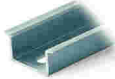
Item no.: 210-197 Steel carrier rail; 35 x 15 mm; 1.5 mm thick; 2 m long; slotted; similar to EN 60715; silver-colored
