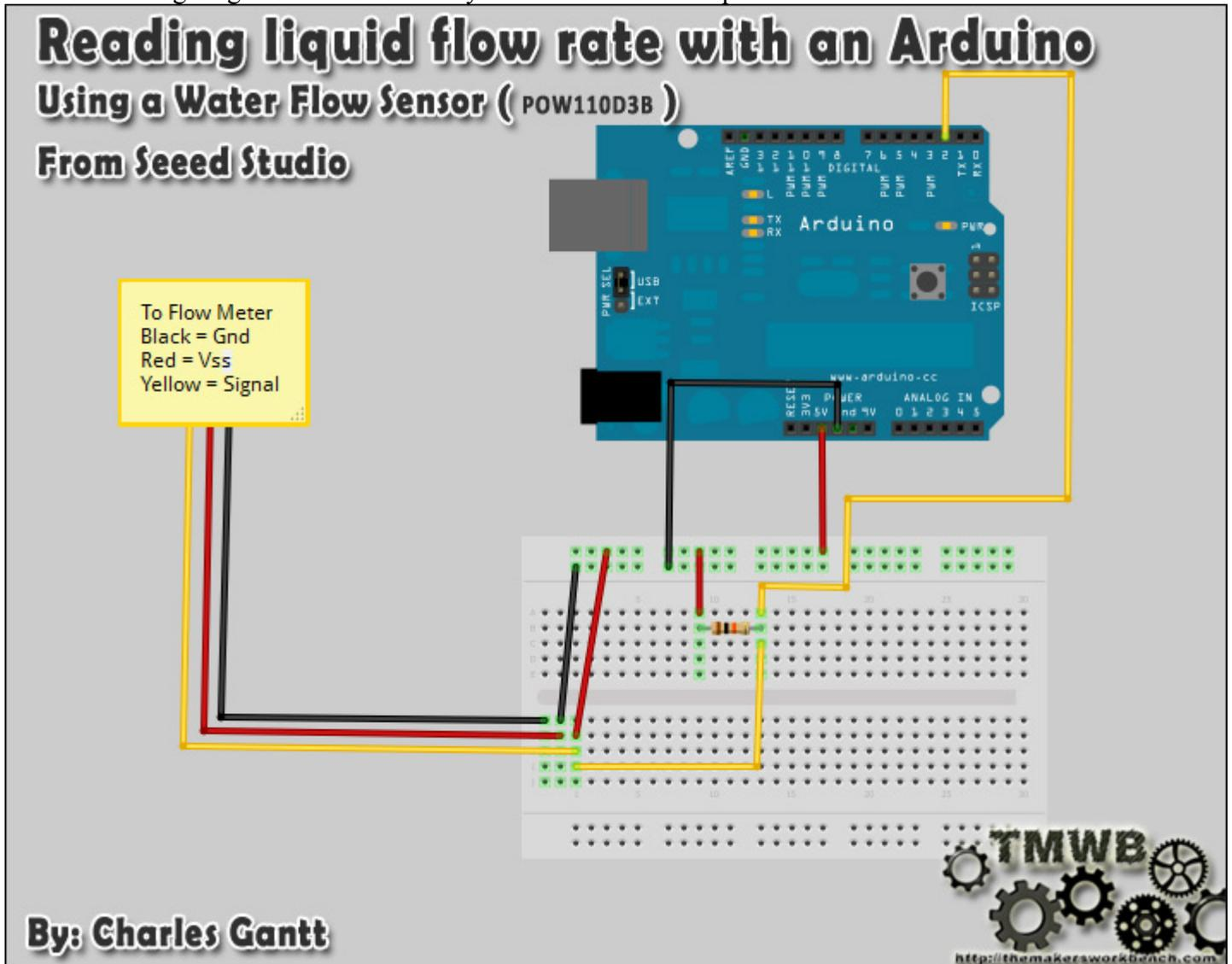
Once you have it wired up you will need to upload the following code to your Seeeduino. Once it is uploaded and you have some fluid flowing through the Water Flow Sensor, you can open the serial monitor and it will display the flow rate, refreshing every second.
