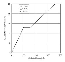
**Figure 6 • Gate Charge Characteristics**
