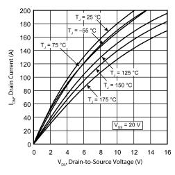
Figure 1 • Drain Current vs. V<sub>DS</sub>
