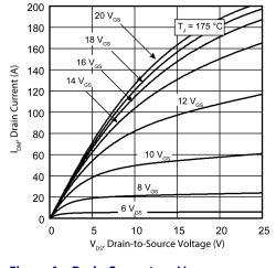
Figure 4 • Drain Current vs. V<sub>DS</sub>
