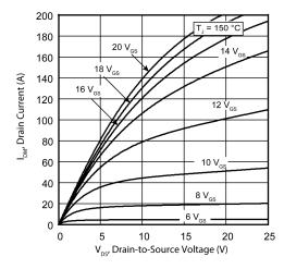
Figure 3 • Drain Current vs. V<sub>DS</sub>
