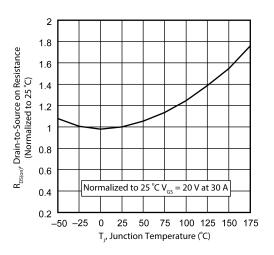
Figure 5 • RDS(on) vs. Junction Temperature
