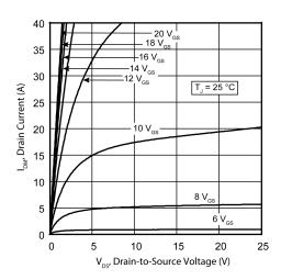
Figure 2 • Drain Current vs. V<sub>DS</sub>
