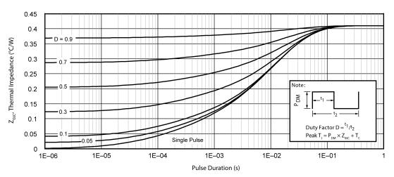
Figure 13 • Maximum Transient Thermal Impedance
