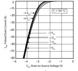
Figure 9 • I<sub>DM</sub> vs. V<sub>DS</sub> 3<sup>rd</sup> Quadrant Conduction
