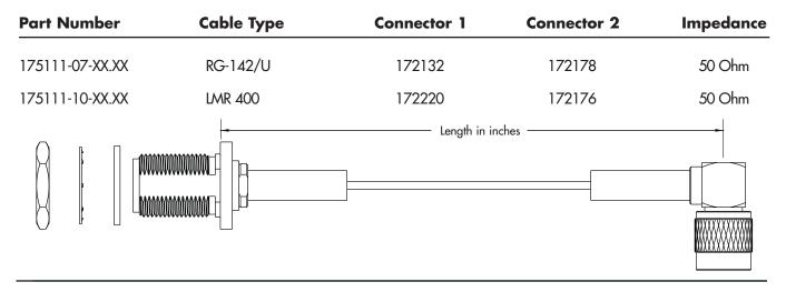
**Amphenol Connex Between Series Cable Assemblies** have different series connectors on each end. Combinations of different series along with different connector styles are offered in a variety of impedances that function at a variety of different frequencies. Each assembly is limited by the lower performing end. Standard lengths are 6, 12, 18, 24, 36, and 48 inches, and custom lengths may also be available. Heat shrink representation may vary.
