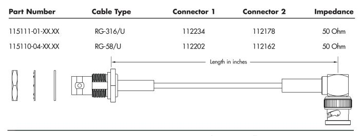
**Amphenol Connex TNC Cable Assemblies** utilize TNC connectors on both ends. TNC connectors are the same physical size as BNC connectors, but feature a threaded coupling mechanism. The 50 Ohm assemblies function up to 11 GHz while the 75 Ohm assemblies function up to 3 GHz. These assemblies are often used in commercial and military antenna applications. Standard lengths are 6, 12, 18, 24, 36, and 48 inches, and custom lengths may also be available. Heat shrink representation may vary.
