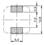
no sensitive traces underneath the component
