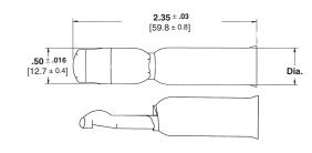
Inside Diameter .516±.005 [13.1±0.13] for 1/0 AWG .512±.005 [13.0±0.13] for 1 AWG, 2 AWG, and 4 AWG
