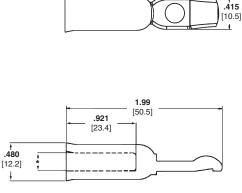
\*Inside Diameter 6 AWG .222 [5.64]; 4 AWG .295 [7.5]; 2 AWG .344 [8.74]
