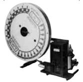
The semiautomatic power applicator is designed to produce a carefully controlled uniform pressure crimp while providing a high rate of production. The applicator features matching dies that fully bottom at the completion of the crimp to provide proper crimp height. The one die set is fully adjustable to provide the full range of crimp heights for all wire sizes.
