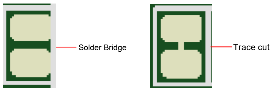
Figure 6-1 Solder Bridge and Trace Cut
