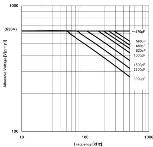
The temperature of the surface of capacitor: below the upper limit of its rated operating temperature range. (including self-heating)
