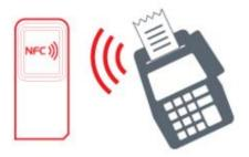
In this mode, NFC click emulates an NFC tag. It doesn't initiate the communication, it only responds to an NFC reader. A typical application of the card emulation mode is how people use NFC in their smartphones to replace several cards, badges and tags at once (using the same phone for tollgate check ins, contactless payments and so on). Card emulation mode, however, is not useful just for smartphones, but for any type of portable device.
