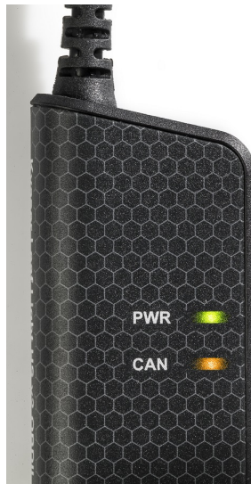
Figure 4: LEDs on the Kvaser Leaf Light v2.
